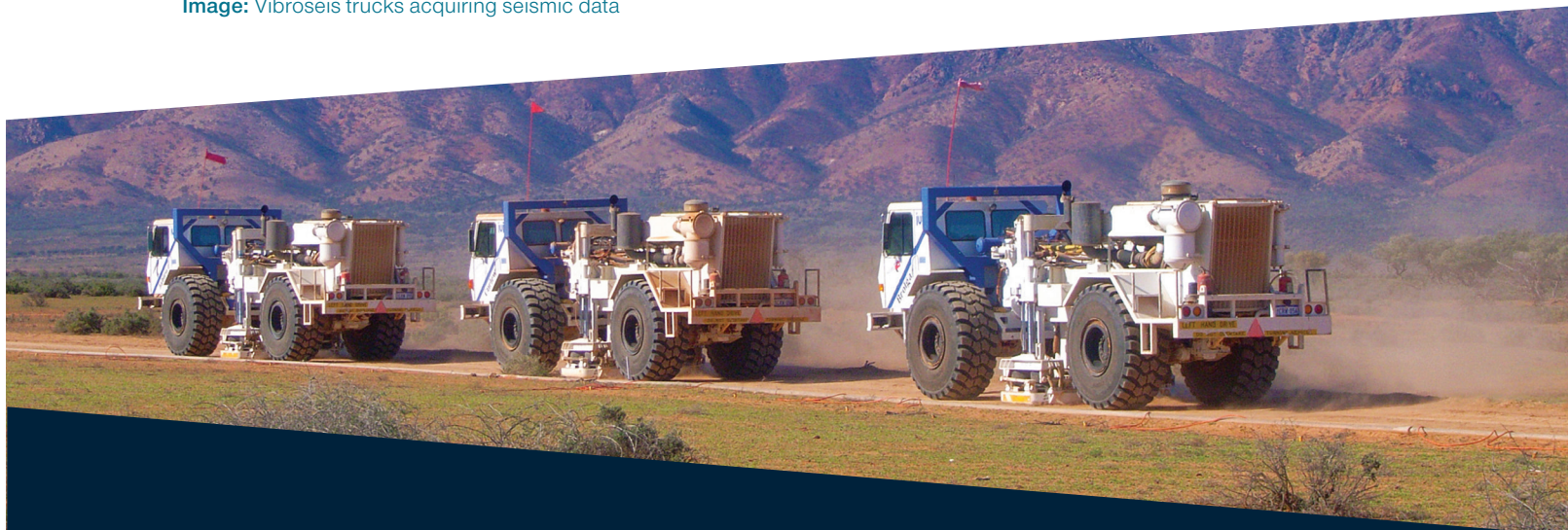
Image: Vibroseis trucks acquiring seismic data
